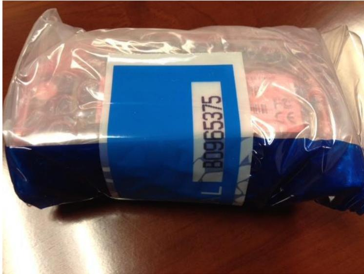
**Figure 1:** POI Device in tamper evident bag with a tamper evident sticker on it
